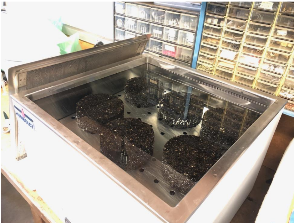
Lottman 140^{\circ}\text{F} ( 60^{\circ}\text{C} ) Conditioning Water Bath
