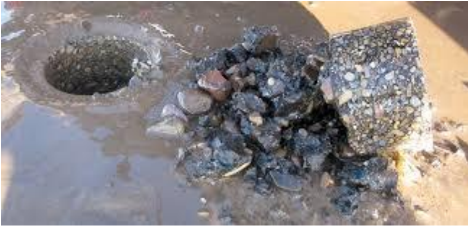
Core with Stripped Layer Below
