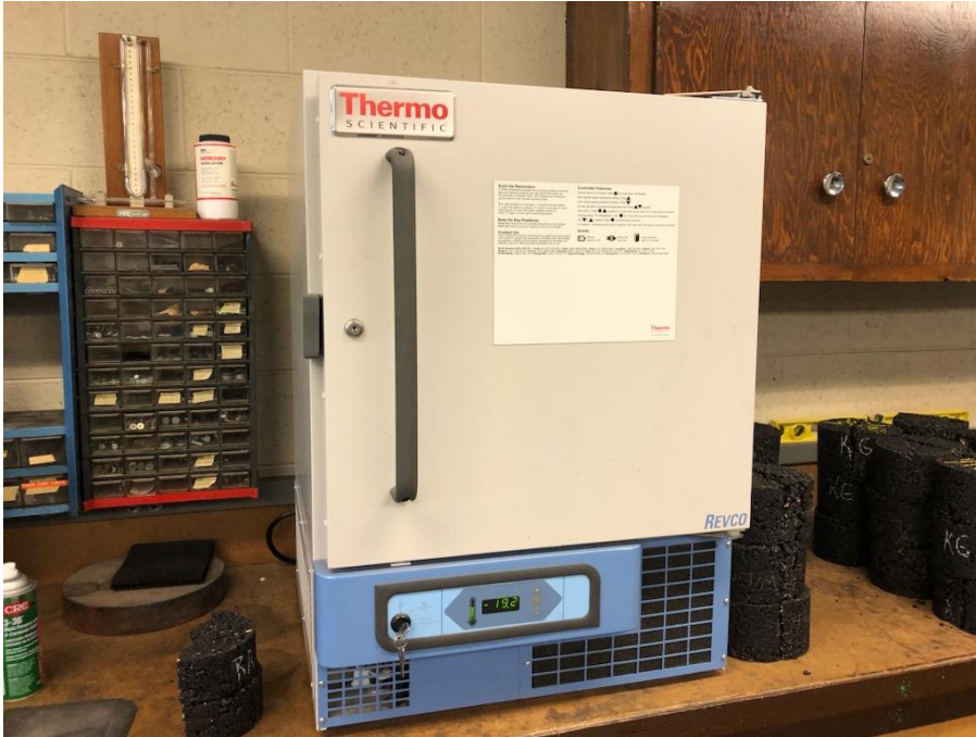
Lottman Conditioning Freezer at -0.4^{\circ}\text{F} ( -18^{\circ}\text{C} )
