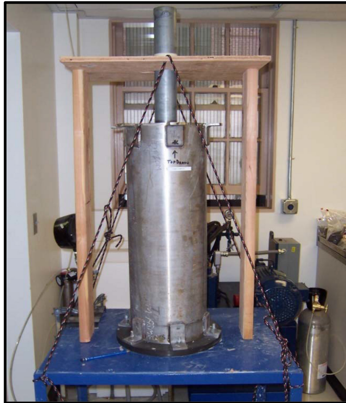
Figure E.2: Sampling Apparatus and Large-Diameter Consolidometer
