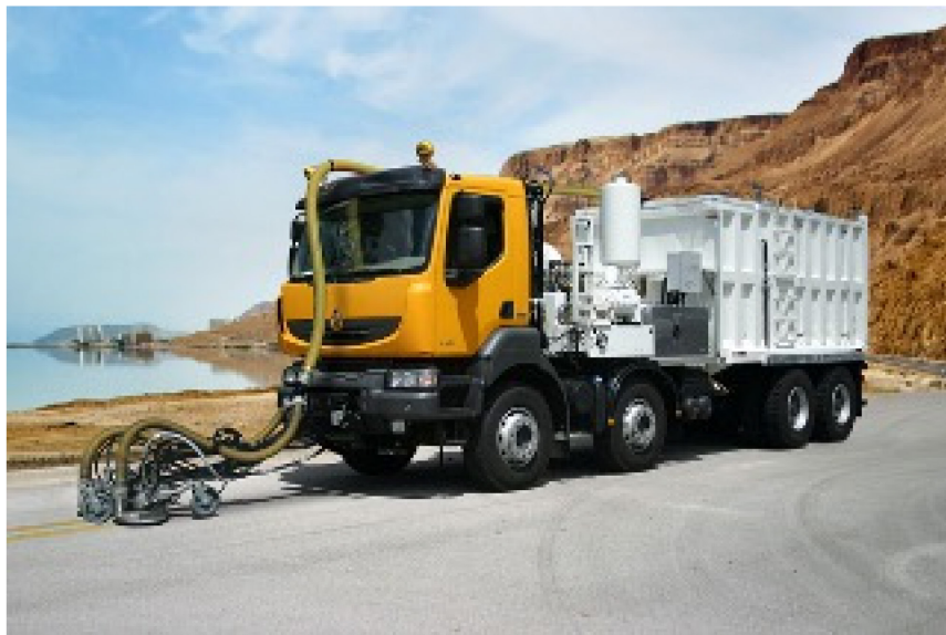
FIGURE 2.2: HIGH-PRESSURE WATER BLASTING TRUCK (GOOGLE, 2021)
