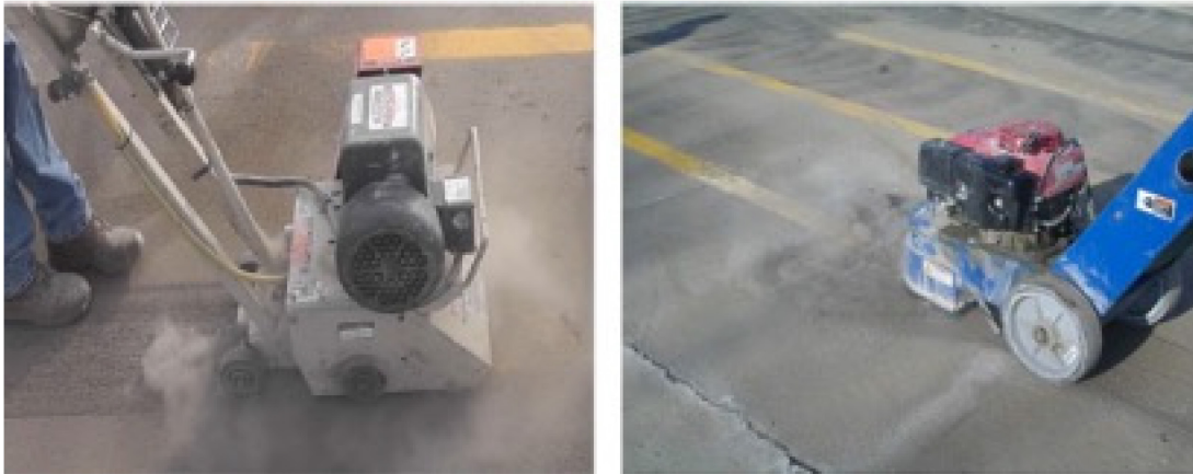
FIGURE 2.3: GRINDER TO THE LEFT AND A SCARIFIER TO THE RIGHT (CHO ET AL., 2013)
