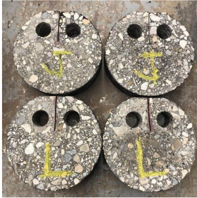
Figure 18. DCT Samples Ready for Testing
