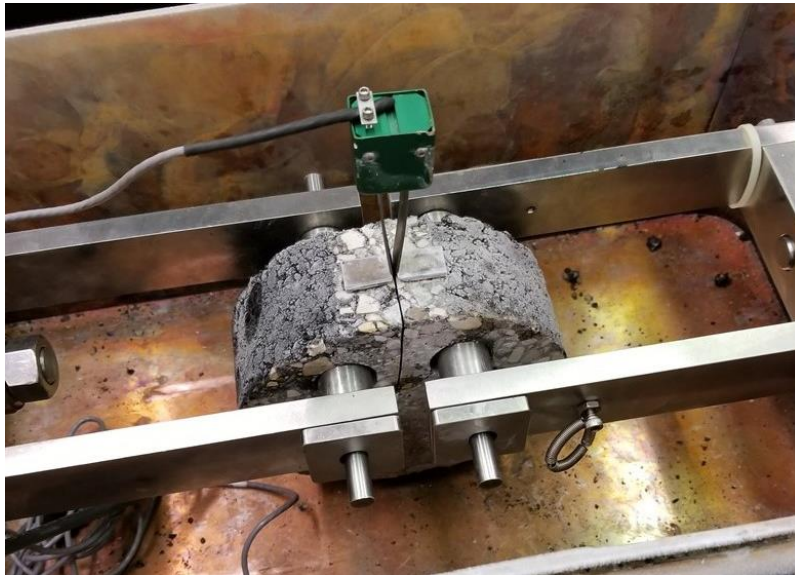
Figure 19. DCT Sample Set-Up
