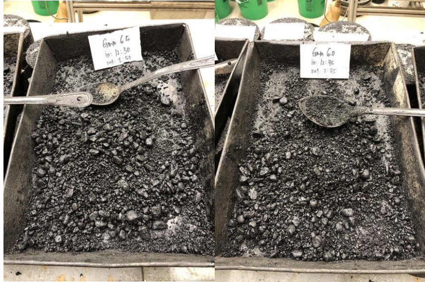
Figure 10. Samples ready for Theoretical Maximum Specific Gravity ( G_{mm} ) testing
