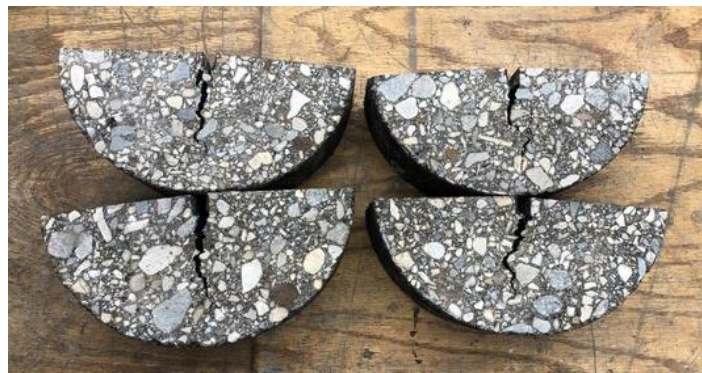
Figure 41. Typical Sample After SCB Test
