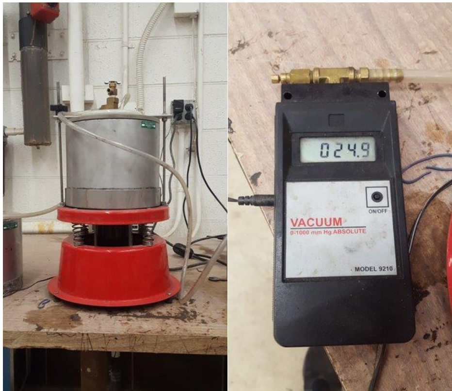
Figure 11. Set-up of bowl and Vacuum Gauge
