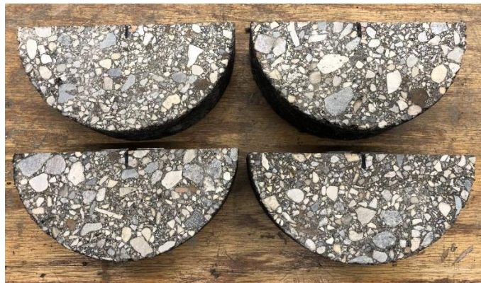
Figure 21. SCB Samples Ready for Testing
