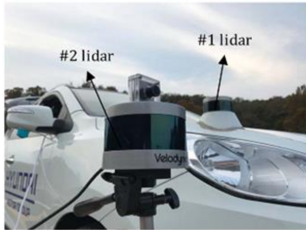
Figure 2.12: LIDAR sensors placed on a Test Vehicle (Kim & Park, 2020b)
