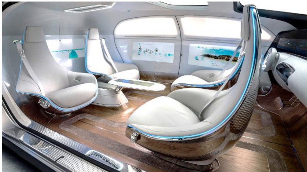
Figure 5.2 SAV interior settings may increase space demands for comfort or work areas, leading to larger and heavier vehicles that consume more electricity thereby raising energy costs.
