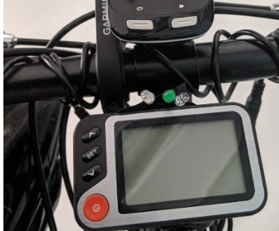
Figure 3.10 Blind spot LEDs mounted on e-bike handlebars to identify obstacles in left, center, and right lanes.
