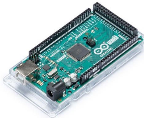
Figure 3.2 Arduino Mega 2560 microcontroller (Arduino 2019a)
