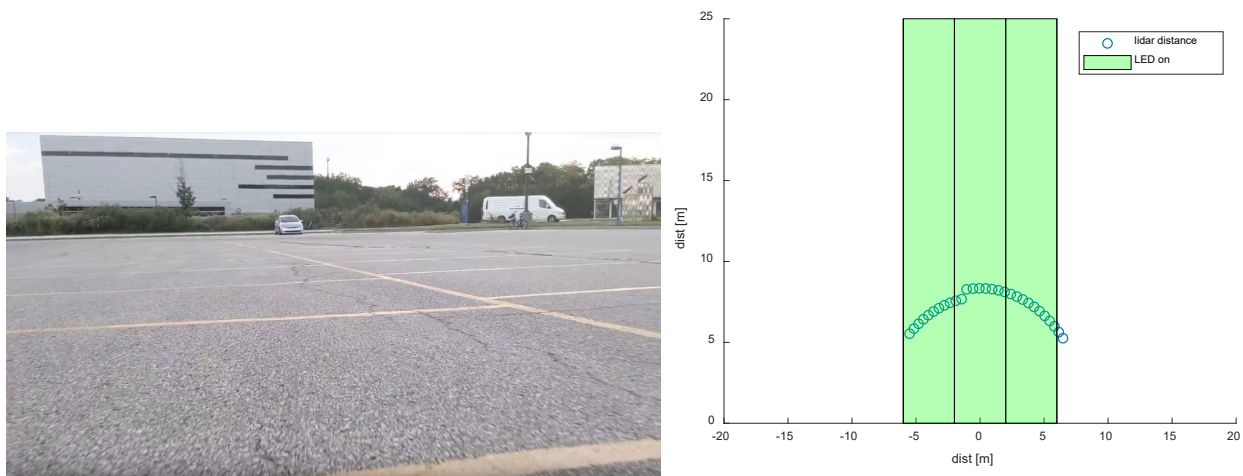
Figure 3.17 Typical visual behind e-bike (left) and sweep data (right) from first mobile test with downward lidar angle
