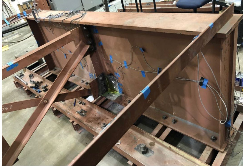
Figure 3.1 Girder subassembly showing the web-gap region
