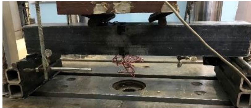
Figure 2.3 Bending test setup
