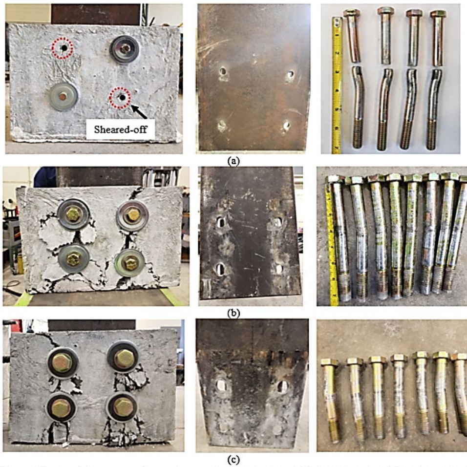
Figure 5.5 Typical failure modes for specimens with (a) \frac{1}{2} in., (b) \frac{3}{4} in., and (c) 1 in. diameter SC
