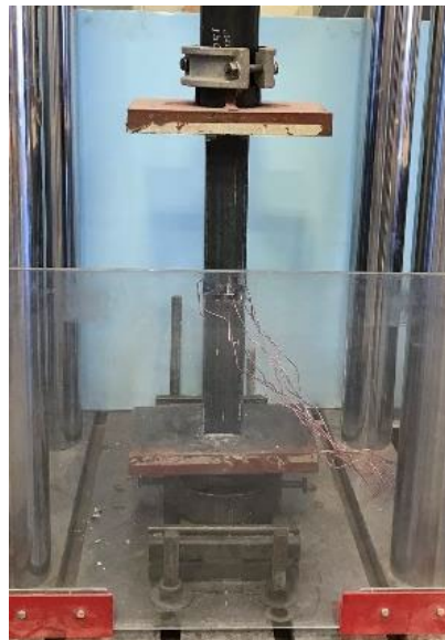
Figure 2.2 Compressive test setup
