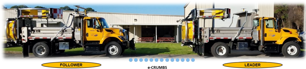
Figure 2.1 Lead-Follower ATMA Vehicle System
