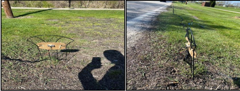
Figure IV.43 - Installing Smraza Ultrasonic sensor along Major Road
