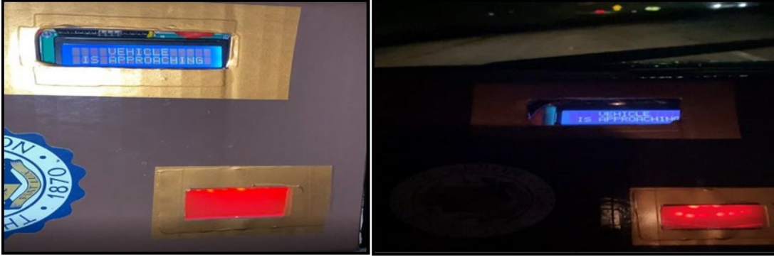
Figure IV.48 - Data Acquisition Unit presenting Three Types of Warnings
