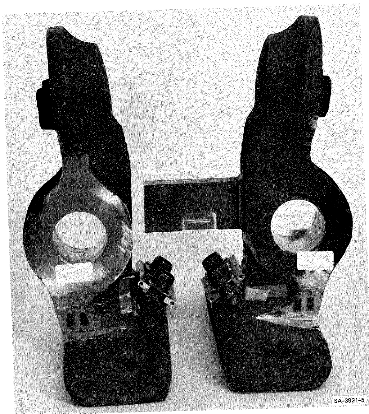
FIGURE IV-3 STRAIN GAGES ON LEVER ARMS
