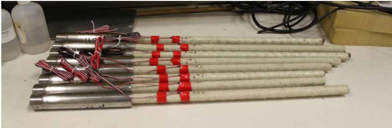
Figure 2.4 Prepared bars with strain gauge installed
