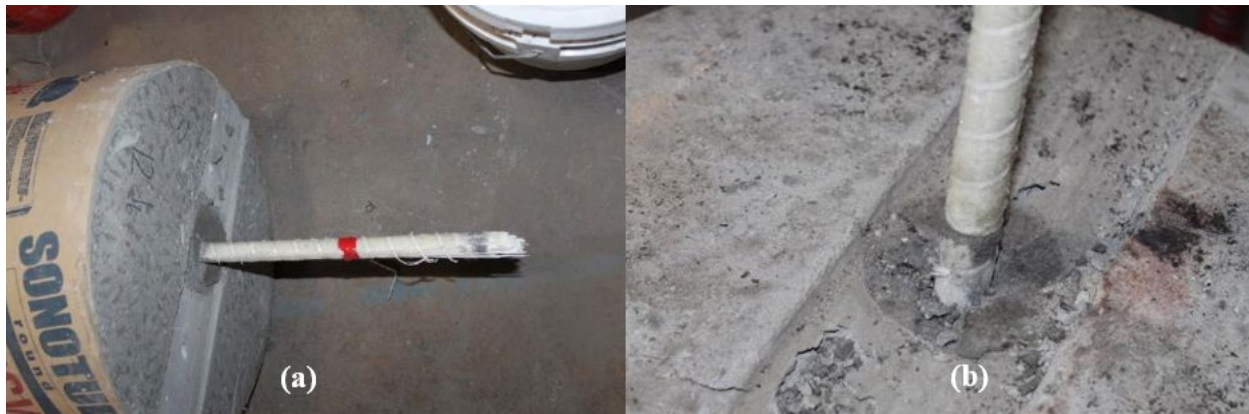
Figure 2.6 Failure modes: (a) bar fractured, (b) bar slipped out, or bar to grout bond failure
