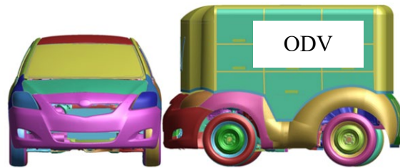
Figure 16. Real-world impact scenario 3 – side crash
