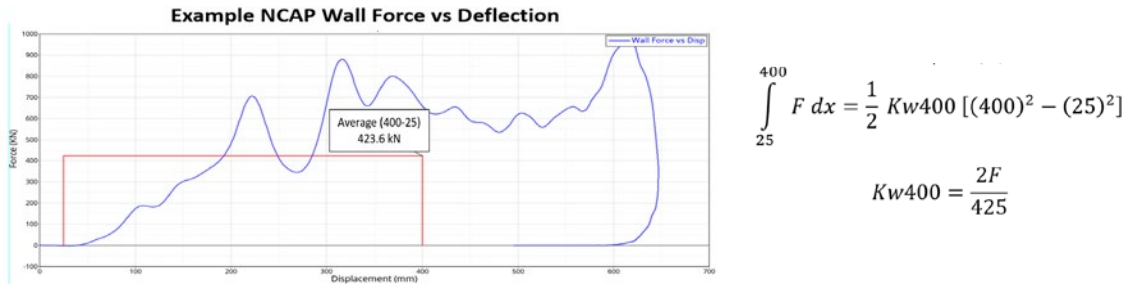
Figure 43. (a) Crush Work Stiffness compatibility metric basis; (b) KW400 equation
