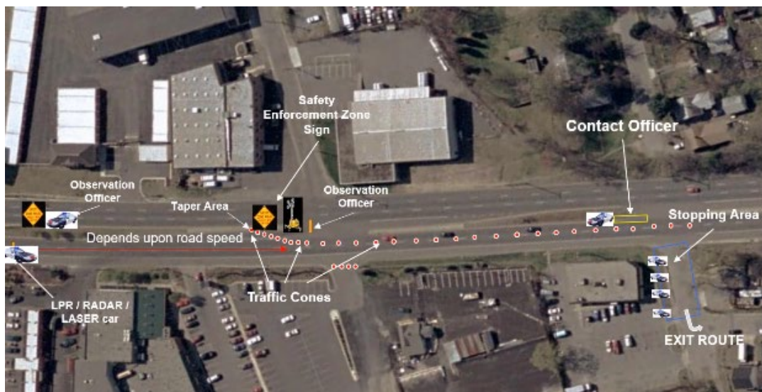
Figure 4. Example site map of safety enforcement zone used by Montgomery Police Department, MD
