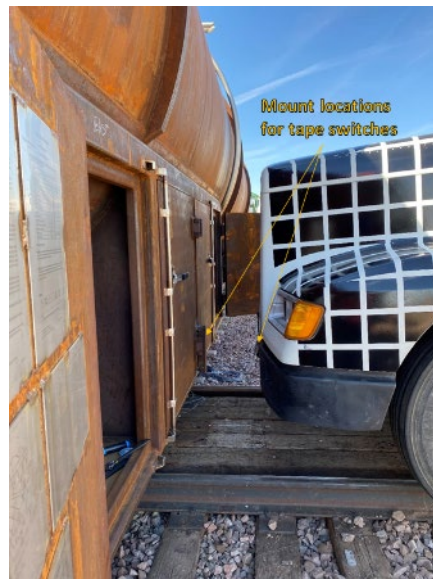
Figure 22. The Dump Truck in Proximity to the LNG Fuel Tender Showing the Mount Locations of the Tape Switches
