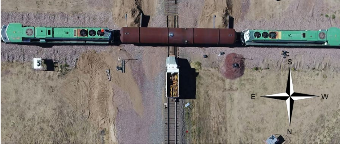
Figure 18. Aerial View of the Test Setup with the Locomotives, Tender and Dump Truck in Position
