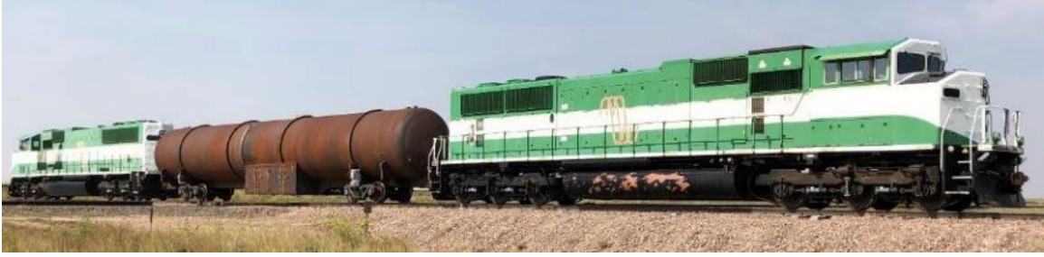
Figure 16. Overview of Test Setup with Locomotives and Fuel Tender
