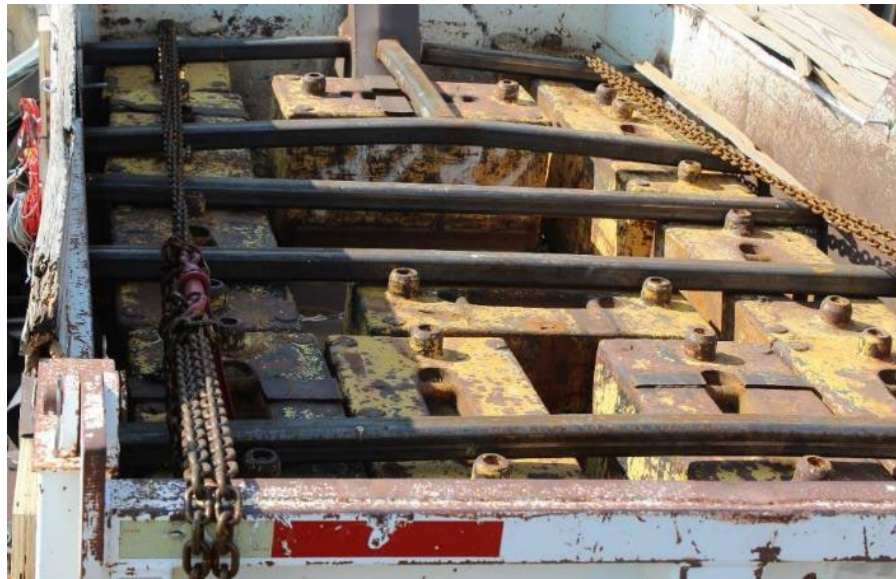
Figure 27. Condition of the Weights and Restraining System Post-Impact
