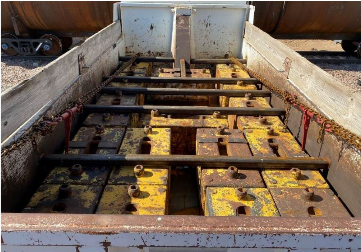
Figure 7. Arrangement of the Dump Truck Bed Loaded with Weights and Restraining System
