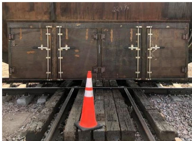
Figure 15. Alignment of the LNG Fuel Tender Housing with the Center of the Track
