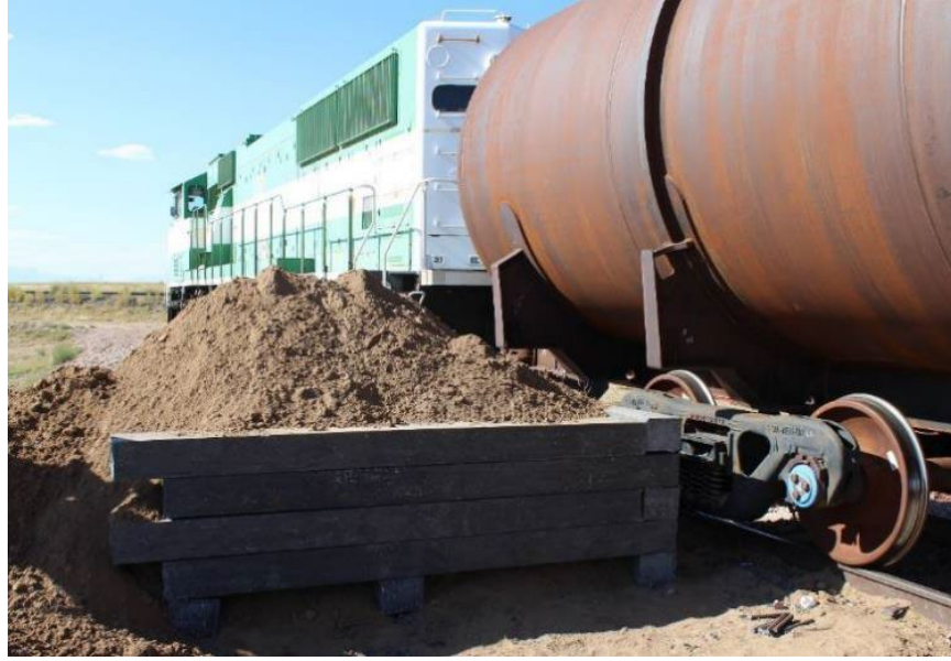
Figure 14. Roll Inhibitor Structure to Prevent Excessive Body Roll of the Fuel Tender after Impact
