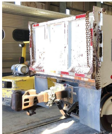
Figure 9. Railway Coupler Fitted to Dump Truck
