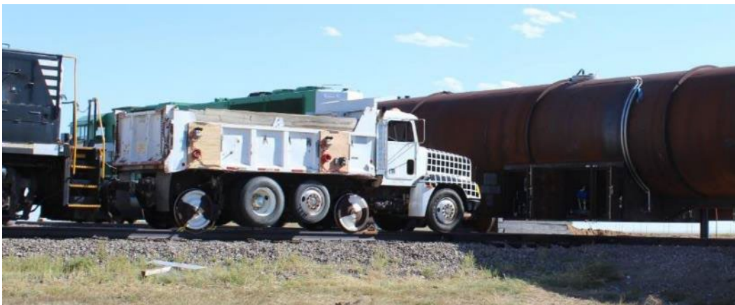
Figure 3. Oblique View of Dump Truck Aligned at the Impact Point with the Tender
