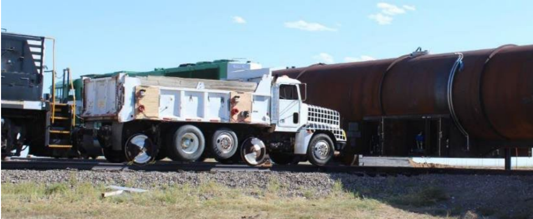
Figure 17. Pre-test Test Setup with Dump Truck Close to the Housing of the Fuel Tender
