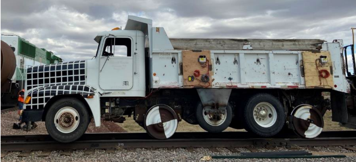
Figure 6. Dump Truck Fitted with the Leaf Spring Suspension and Railway Wheelset
