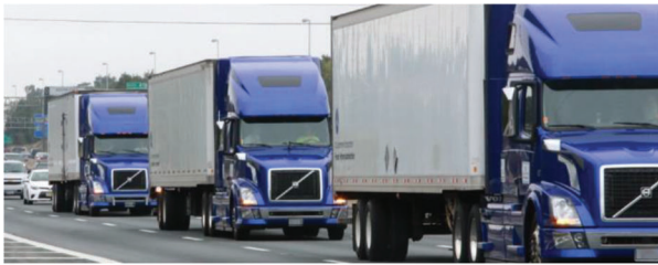
(a) Testing on in-service road (Peloton test) (FHWA, 2021)
