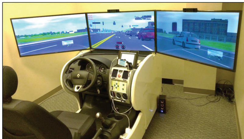
Figure 4.2 Cockpit of the Purdue driving simulator used for the experiment.
