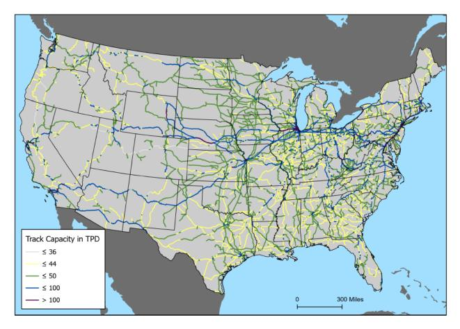
Figure 8. Track Capacity before Adjustment<sup>43</sup>
