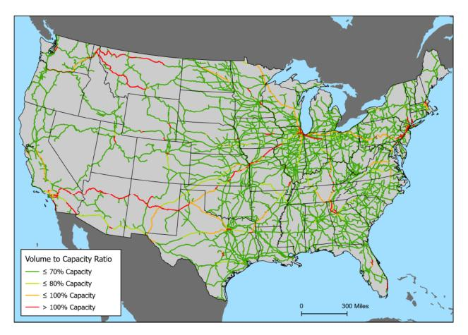
Figure 7. Traffic Volume to Track Capacity Ratio<sup>42</sup>
