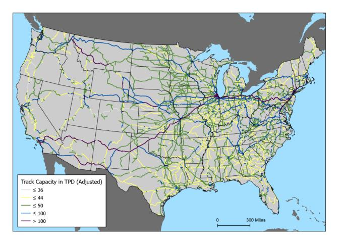
Figure 9. Track Capacity after Adjustment<sup>44</sup>
