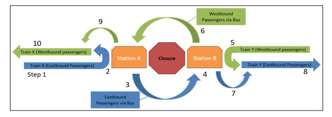
Figure 14. Overview of Bus Bridge Concept for Intercity Passenger Service
