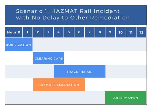
Figure 2. Gantt Chart of Possible Delay Scenario One for a HAZMAT Incident
