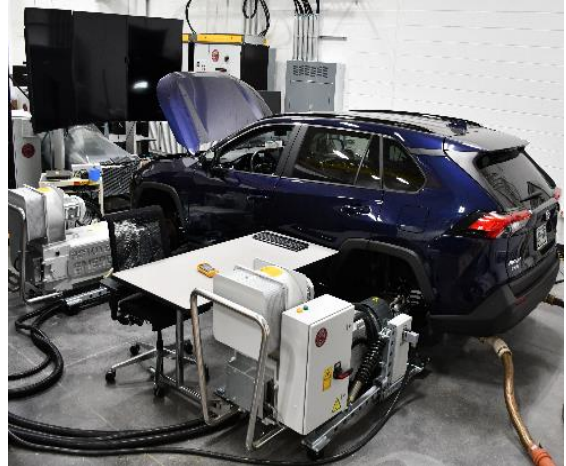
Figure 12: The RotoTest simulator featuring vehicle mounted on a steerable dyno with virtual sensors has been commissioned and it is ready for testing. (Source: Shean Huff, Oak Ridge National Laboratory)
