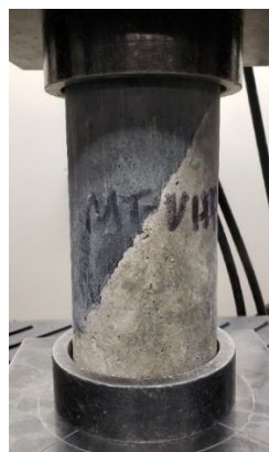
Figure 30: Slant-shear specimen in load frame
