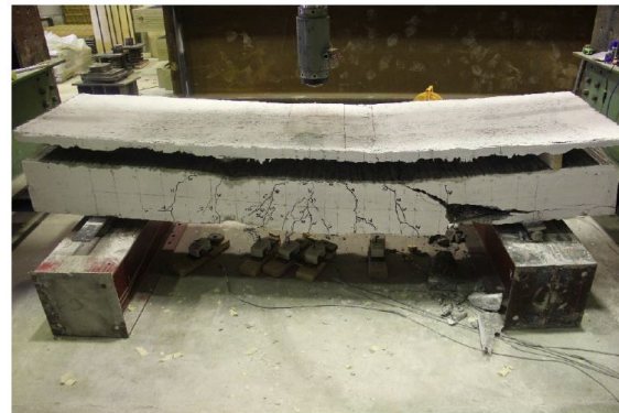
c) UHPC layer pried open after the test
