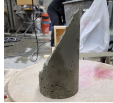
Figure 28: Typical substrate concrete half cylinders for slant shear specimens
