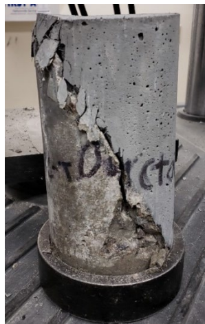
Figure 35: One specimen with a slant shear failure at the bond (Ductal-T 1)
