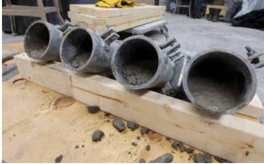
Figure 28: Typical substrate concrete half cylinders for slant shear specimens
