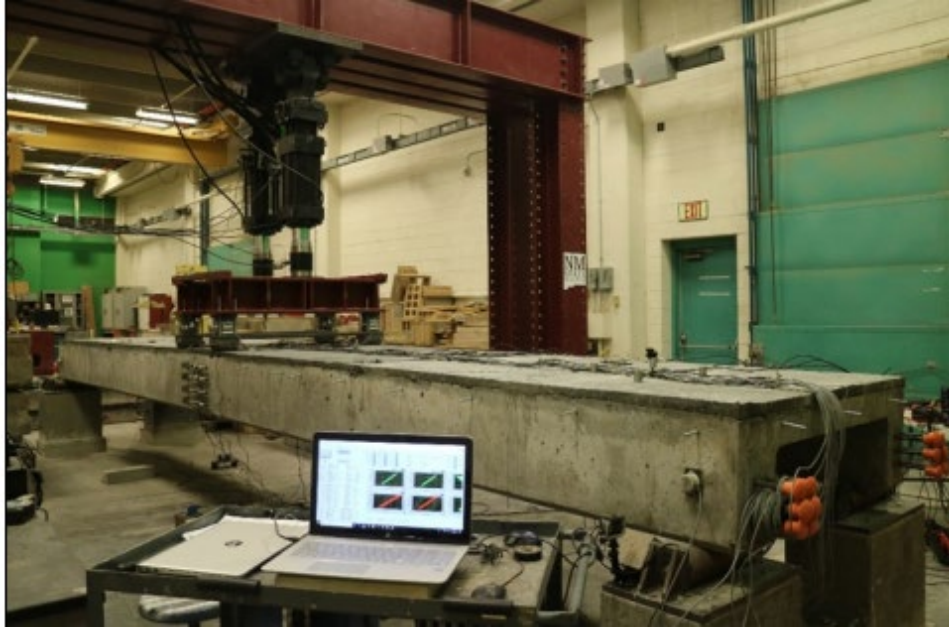
Figure 7: Channel Girder with UHPC overlay [24]
