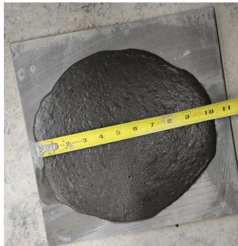
Figure 18: MT-UHPC static flow test
