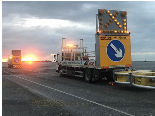
Figure 6. Photo of Automated TMA.
