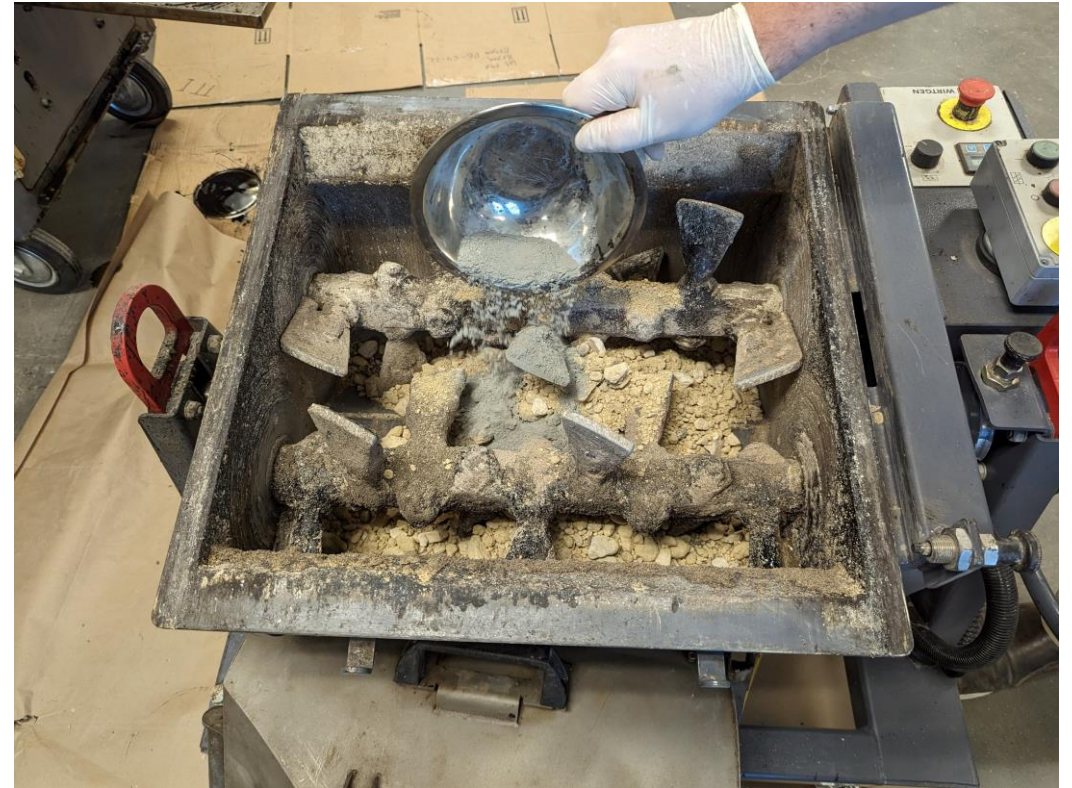
Adding Cement into Material for Mixing Using a Mechanical Mixer
