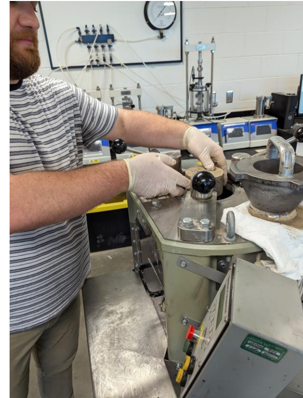
Extruding a 4×2 IDT Strength Test Specimen
