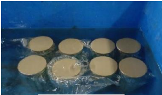
(a) Standard curing in water
