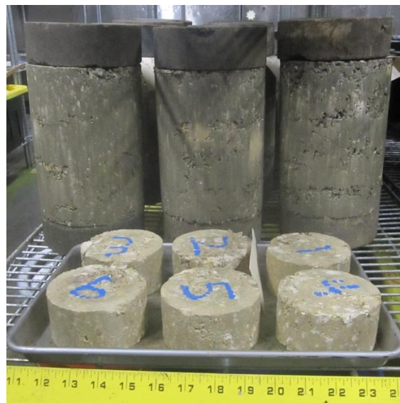
Figure 25. Representative IDT (Front) and UCS (Back) Test Specimens.
