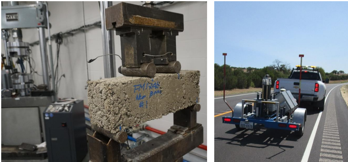
Figure 44. Most Reliable Inputs for CTB Mechanistic Check Include Lab-Measured MoR Values (Left) and Field-Measured FWD Mr Values (Right).
