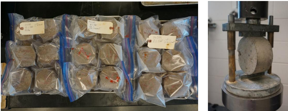
Figure 51. IDT 3 Test Specimens Curing (Left) and being Tested (Right) for Rapid CTB Mix Design.
