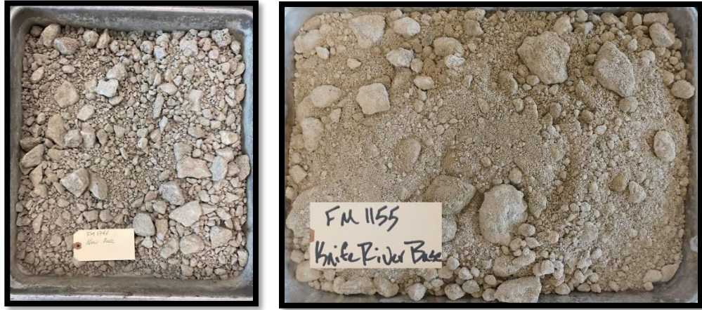
Figure 6. FM 1746 Type A, Grade 1-2 Flexible Base (Left) and FM 1155 Crushed Concrete (Right) Materials Sampled from Stockpile.
