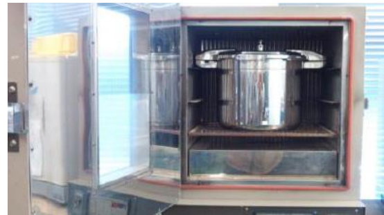
(b) Accelerated curing in pressure cooker and oven
