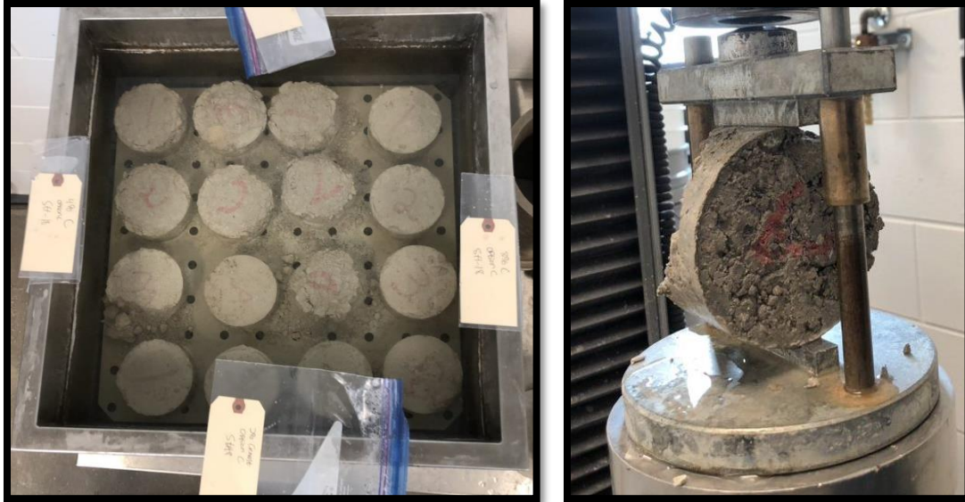
(a) Deteriorated specimens during soaking (b) Significant deterioration of testable specimens
