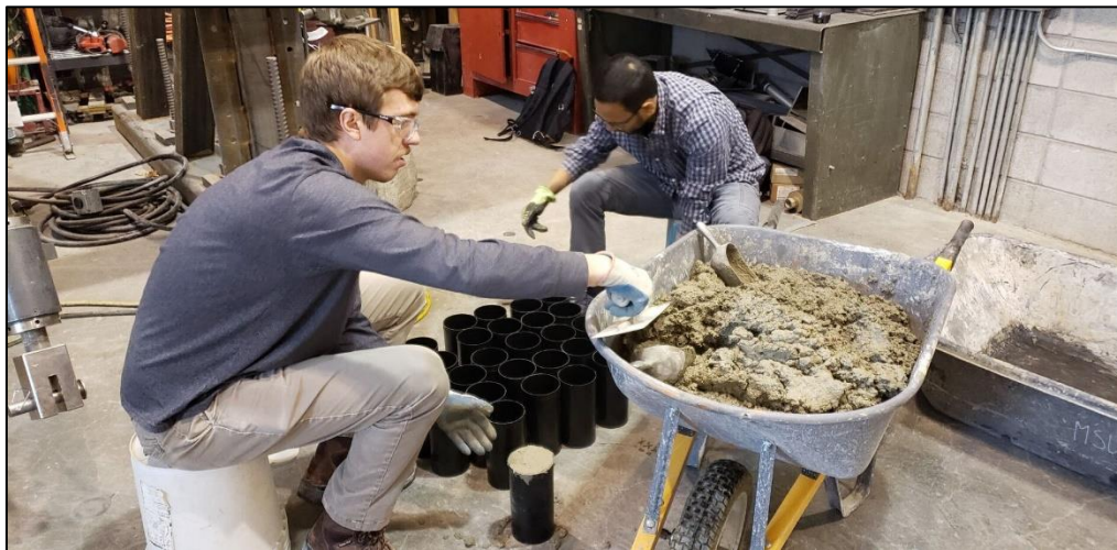
Figure 22: Casting concrete cylinders
