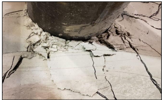
Figure 36: VT2/3-4 concrete crushing on front of pile at failure from initial loading direction
