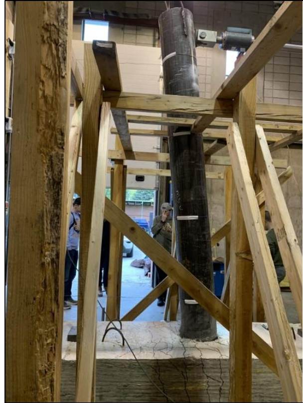
Figure 52: VT2/3-4U failure from reverse push direction
