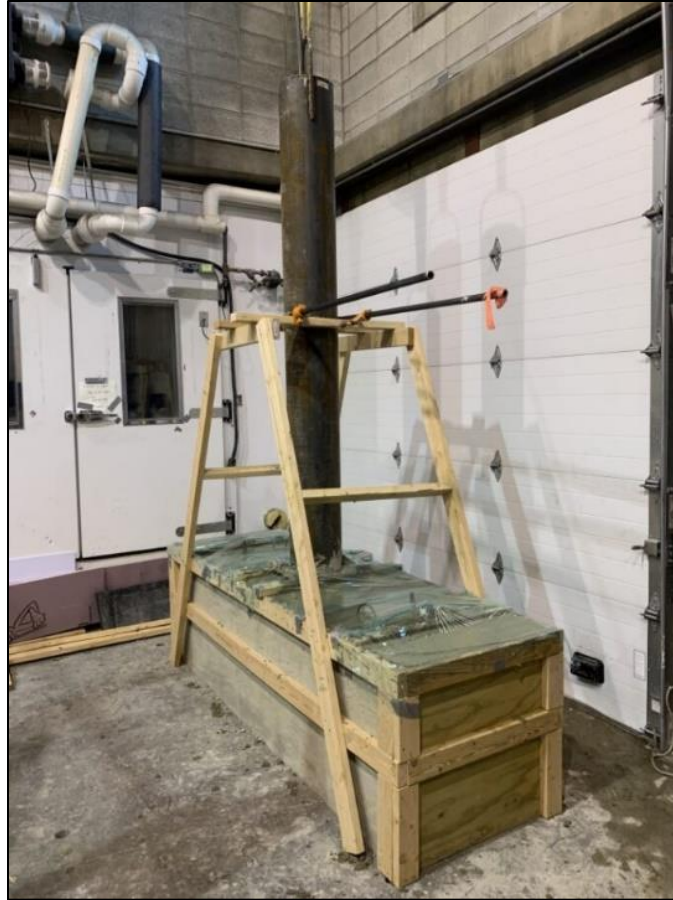
Figure 23: Specimen upon completion of concrete pour
