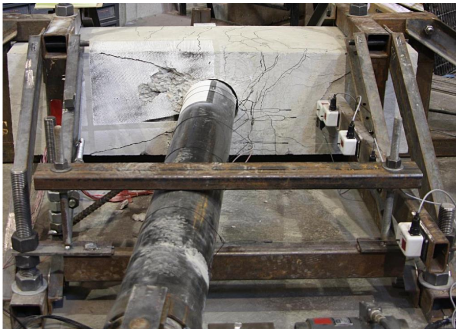
Figure 6: Typical Test Specimen from Previous MSU Research Near Ultimate Load
