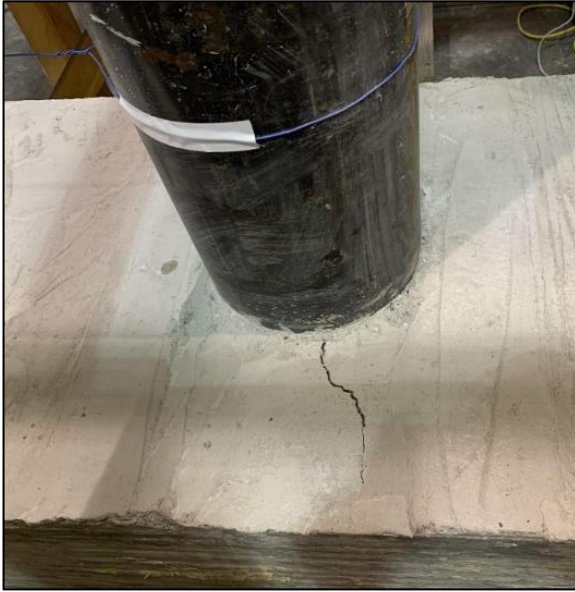
Figure 47: VT2/3-4U first cracks (92 k-ft)
