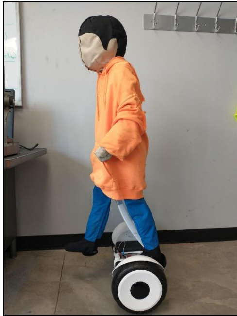
Figure 1: XBot Platform with Pedestrian Soft-Body Proxy
