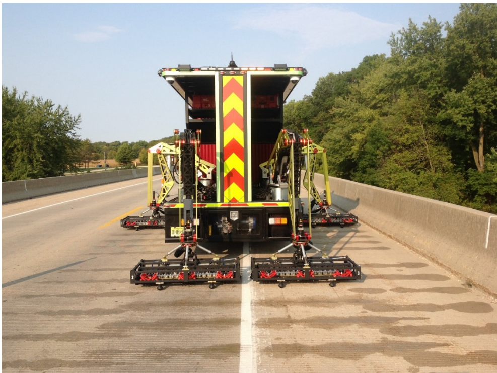
Figure 2 - HD System Collecting Data on a Bridge in Iowa
