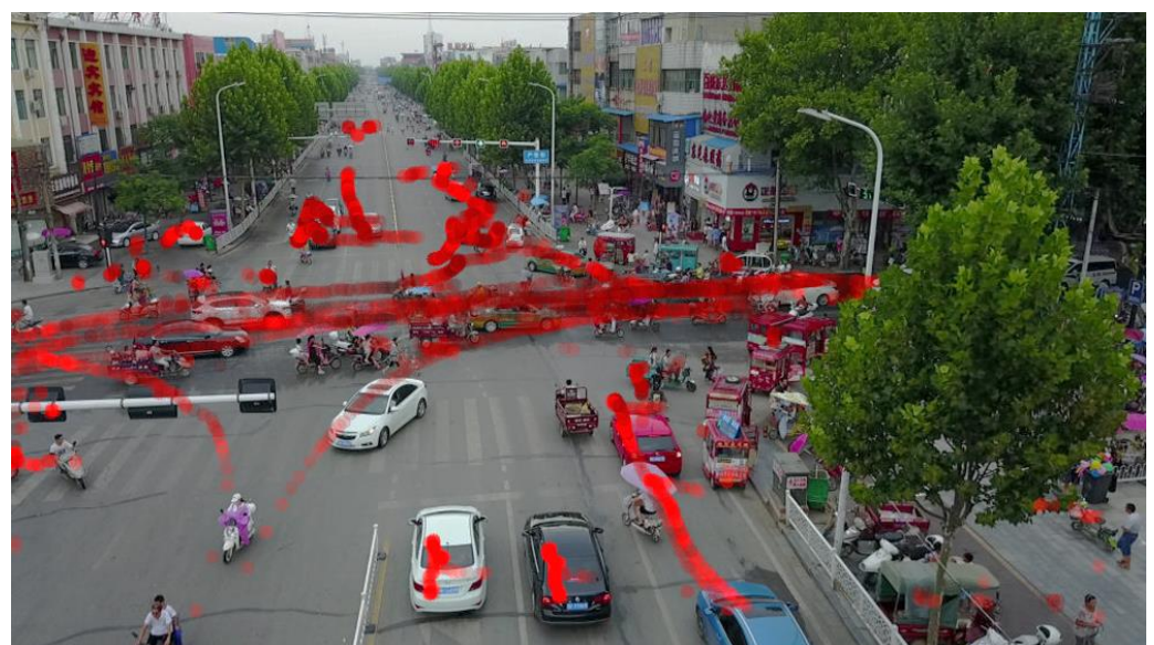
Figure 10. Summary of locations of all interactions where potential collisions could occur. A deeper color indicates a less safe interaction (i.e., a smaller TTC) between road user pairs.
