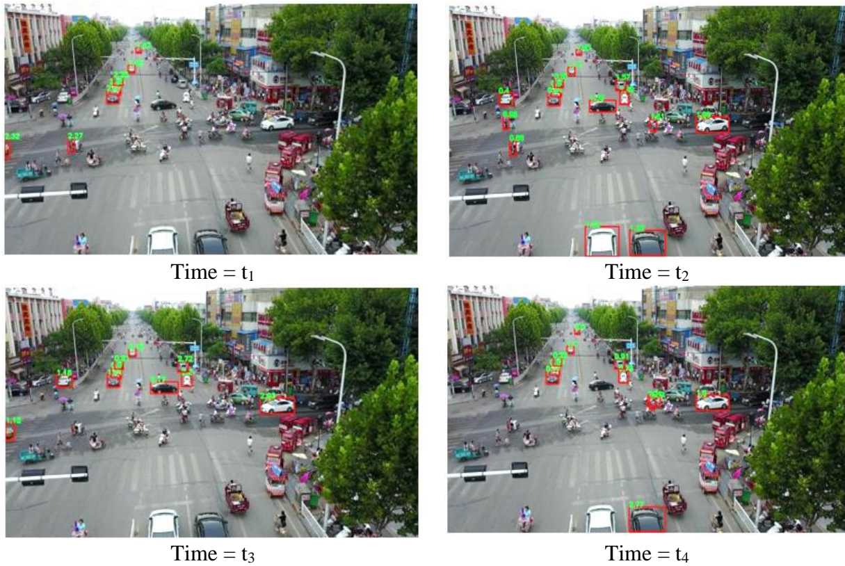
Figure 2.8 Macroscopic risk profile (“risky” road users are marked with red boxes and the number indicated above each box is their smallest TTC value)
