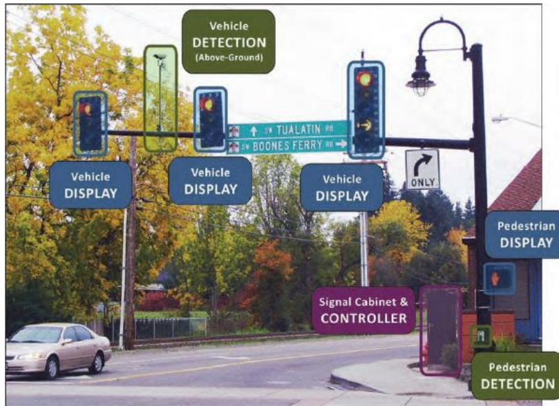
Figure 2.1: Typical Signalized Intersection Components [6]
