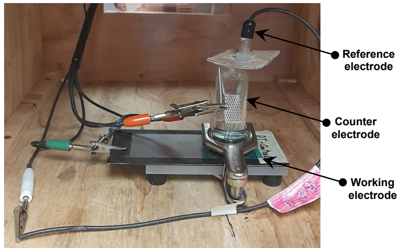
Figure 5-9: Potentiodynamic polarization test set-up for measuring corrosion current densities for MSP coatings.
