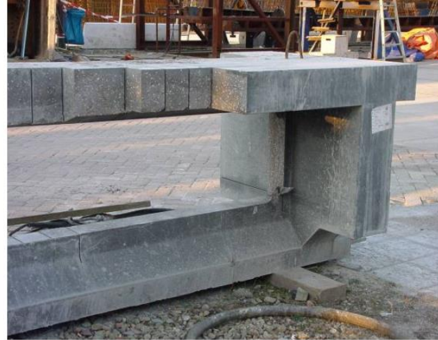
Figure 2.7 (a) General view of one of the Bourg-Les-Valence Bridges, France (Valente 2017); (b) mock-up of one half of a \pi -shape beam before and after sawing (Simon et al. 2013).
