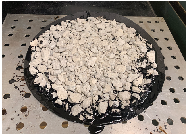
Otta seal specimen showing aggregate rolled into asphalt binder
