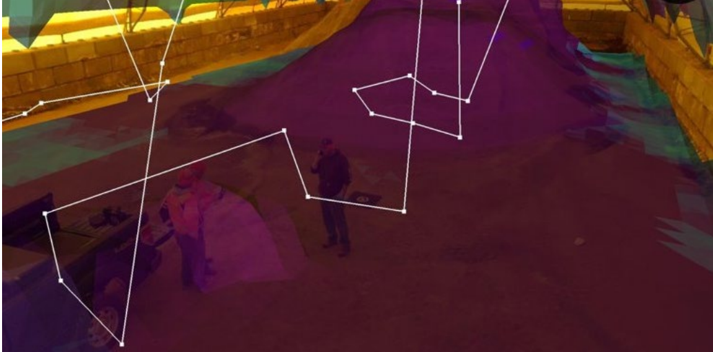
Figure 2. UAS Data Collection Mission within a WYDOT Materials Shed (Source: WYDOT)
