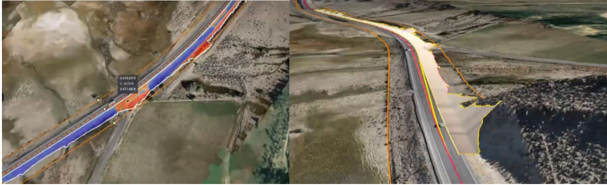
Figure 10. UAS-Collected Data used for Jensen Lane Project Analysis (Source: UDOT)
