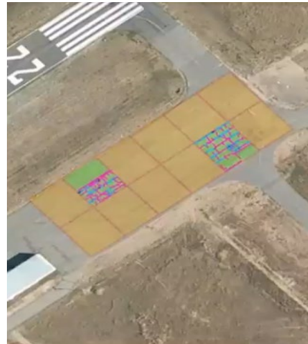
Figure 23. UAS Pavement Inspection of Airport Taxiway(Source: UDOT)
