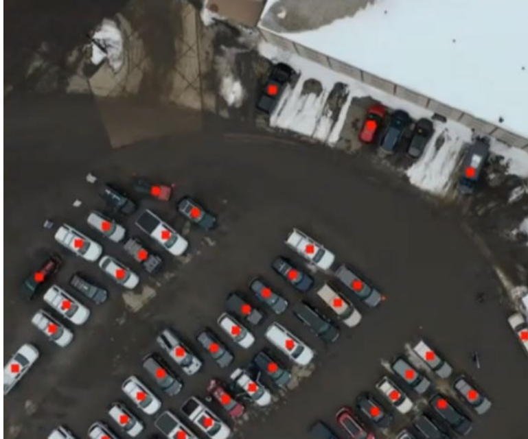
Figure 25. UAS and AI Monitoring Parking Availability(Source: UDOT)
