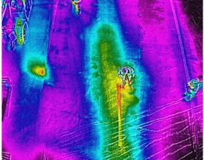
Figure 19. UAS Thermal Analysis of UDOT Bridge Deck. (Source: UDOT)
