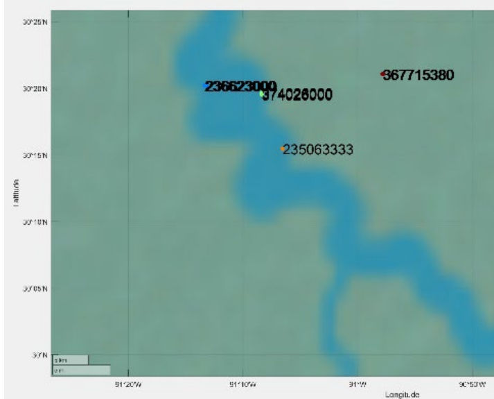
Figure 15: MATLAB Geosscatter plot zoomed to the Mississippi River, including MMSIs to identify vessels.
