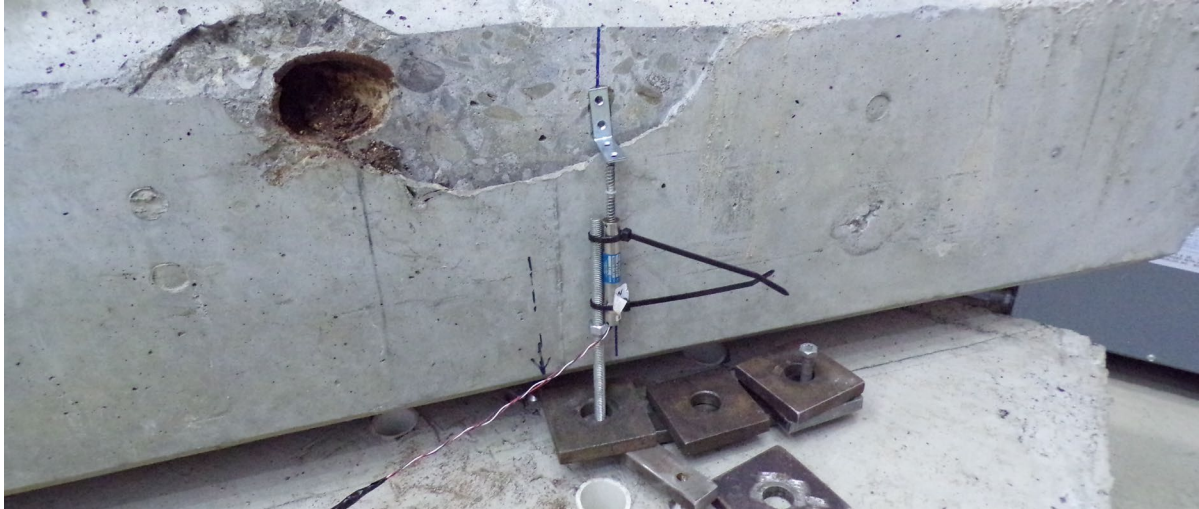
Figure 5.4: Typical attachment of potentiometer at supports
