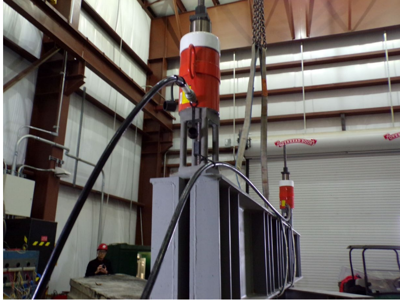
Figure 5.1: Loading beam assembly
