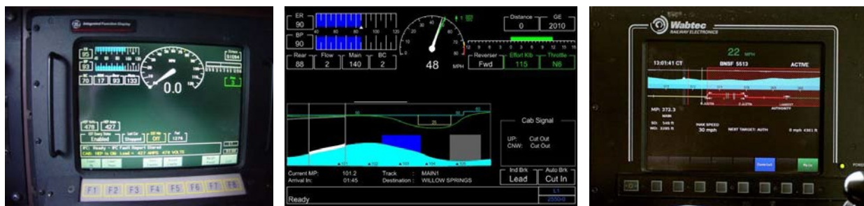
Figure 37. Examples of typical digital locomotive displays. Left: Example of a primary driving display. Center: Trip Optimizer display screen (Wabtec); Right: i-ETMS (Wabtec) PTC display screen. Note that the secondary system displays (TO and i-ETMS) also show primary driving information along with unique system information.
