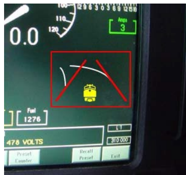
Figure 40. Icon representing an incorrectly lined switch; the intended travel path is to cross over to a new track
