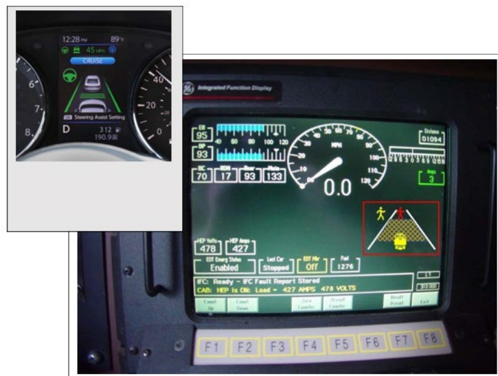
Figure 38. Example of Exp-L symbology on a typical primary operating display; this symbology indicates an obstruction on the tracks (red figure) and another close to the tracks on the left side (yellow figure)
