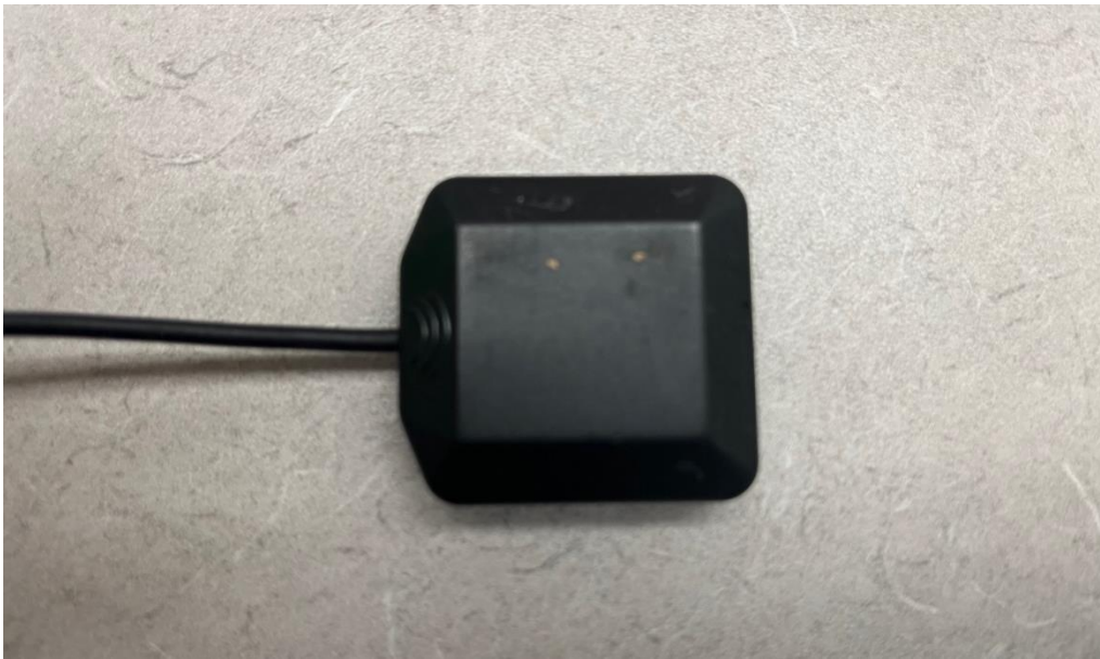
Figure B4. Antenna for GPS module
