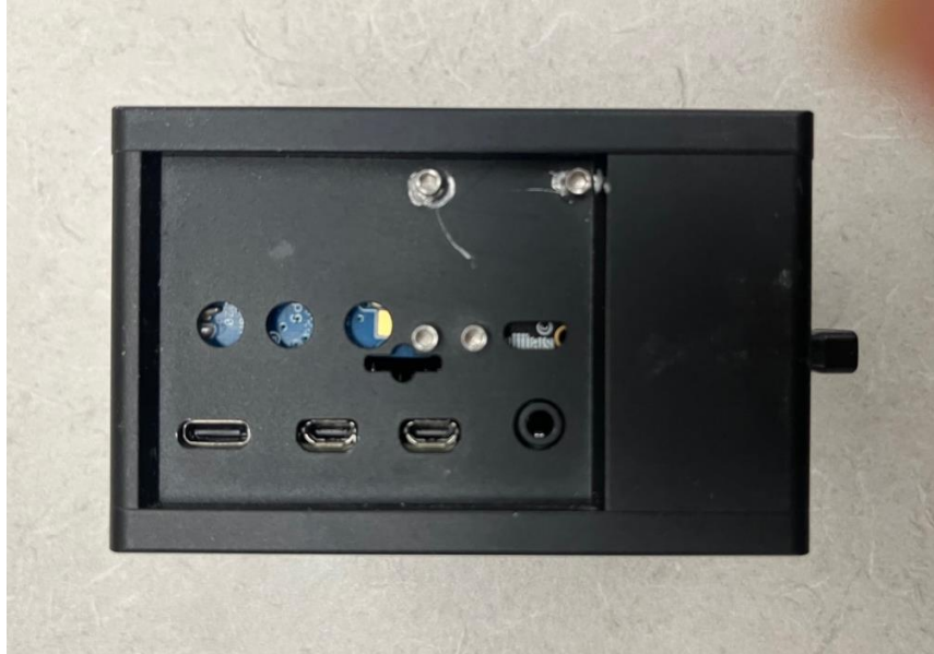
Figure B2. Power interface on the smart box, with the bottom left for USB type-C
