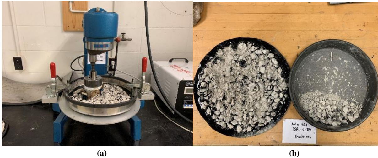
Figure 27. Sweep test: (a) conducting sweep test on Otta seal specimen and (b) collecting loose aggregate after sweep test
