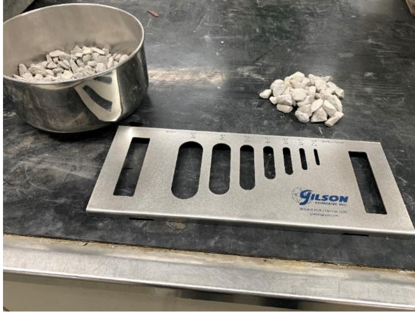
Figure 22. Measuring the average least dimension of aggregate using a thickness gauge
