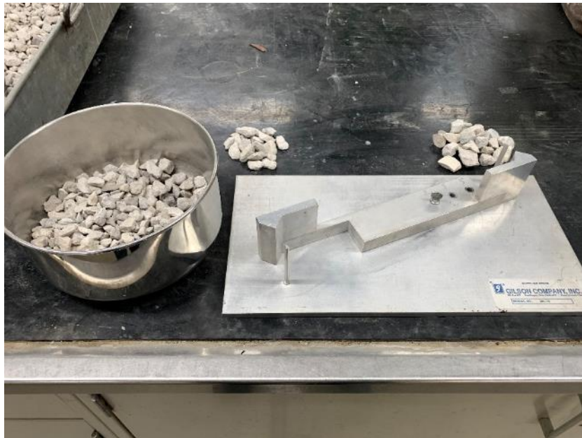
Figure 21. Measuring the flakiness index of limestone aggregate by following ASTM D4791
