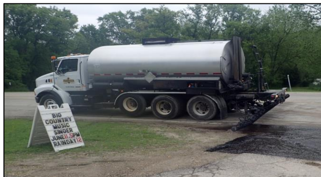
Figure A2. Asphalt distributor
