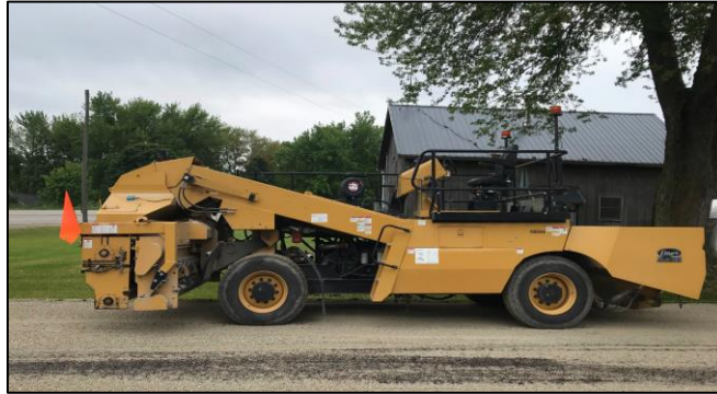
Figure A3. Aggregate spreader
