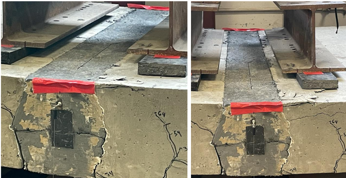
Figure 7.13: Concrete crushing of specimen 2
