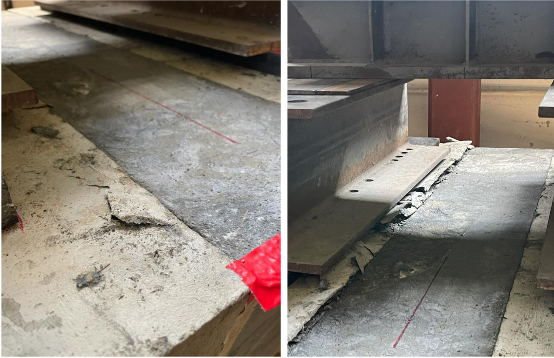
Left: 48 kips, Right: maximum load Figure 7.8: Concrete crushing of specimen 1
