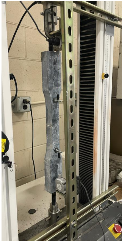
Figure 5.9: Test setup of direct tension test
