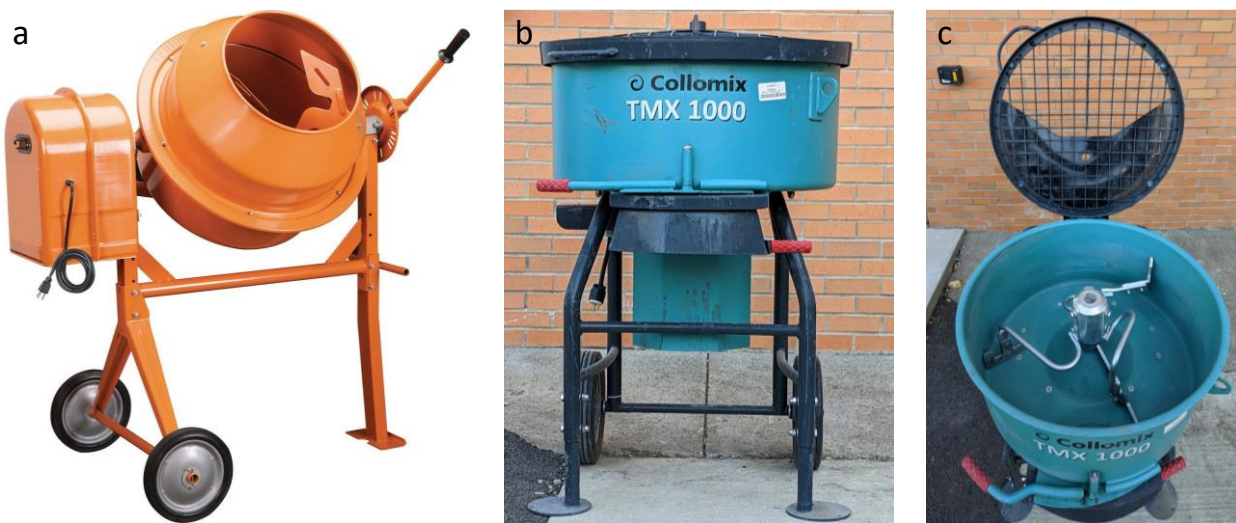
(a) regular drum concrete mixers, (b) and (c) pan mixers
