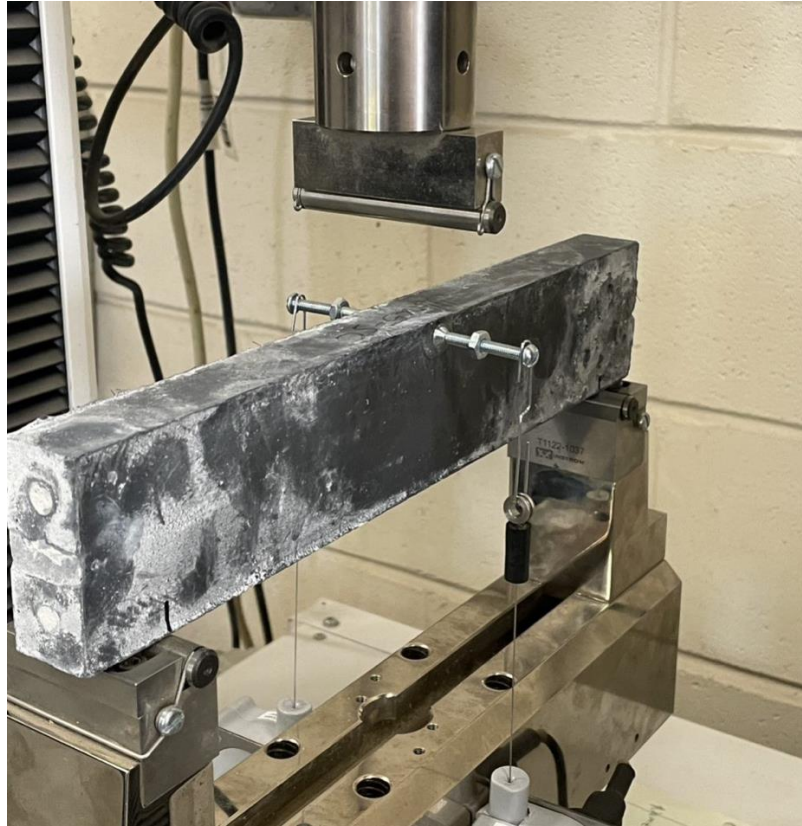
Figure 5.5: Flexural test setup
