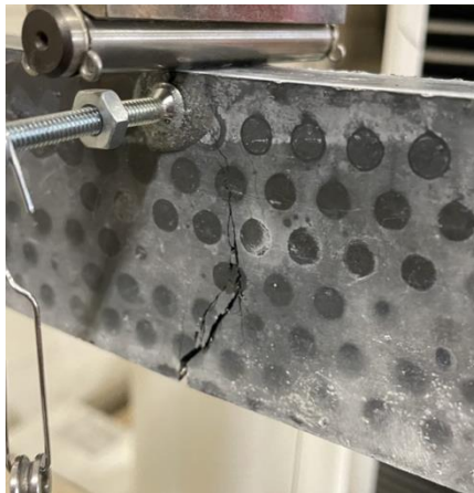
Figure 5.28: Crack in UHPC beams under flexure loading
