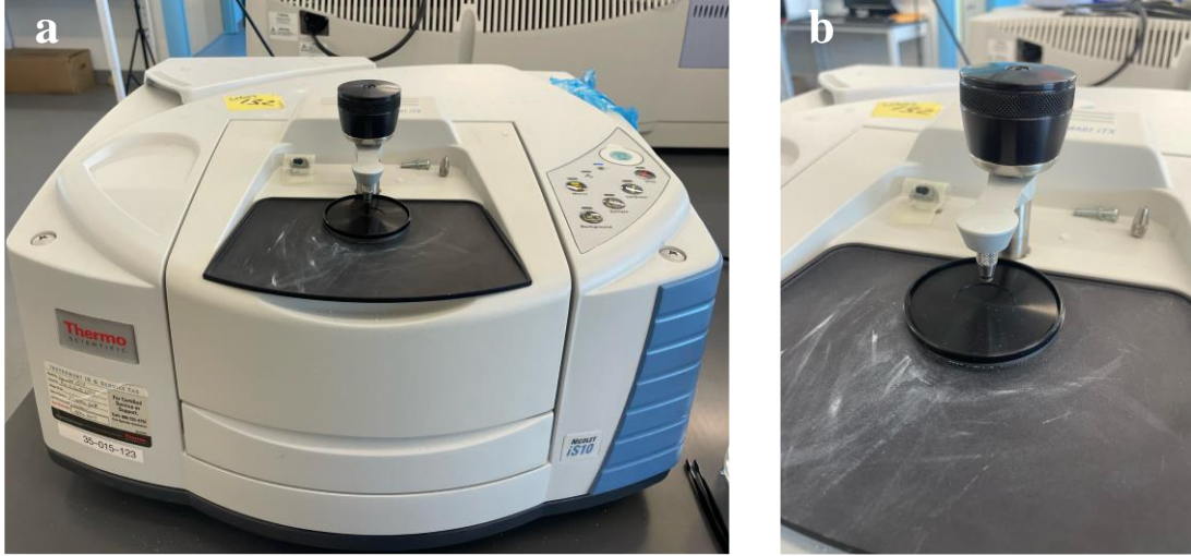
Figure 4.15: FTIR Spectroscopy testing setup.
