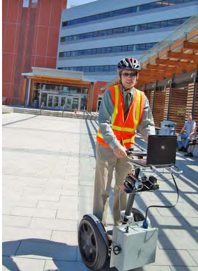
(a) ULIP- Ultra Light Inertial Profiler for sidewalk evaluation (Photograph from https://www.corada.com/products/starodub-inc-ultra-light-inertial-profiler-ulip-for-sidewalks )
