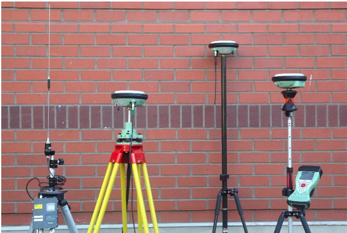
Figure 2.6: GNSS receivers mounted in different configurations.
