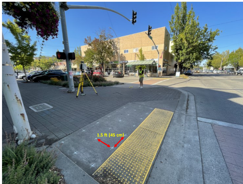
Figure 7.3: Example sampling grid marked with chalk for slope measurements.
