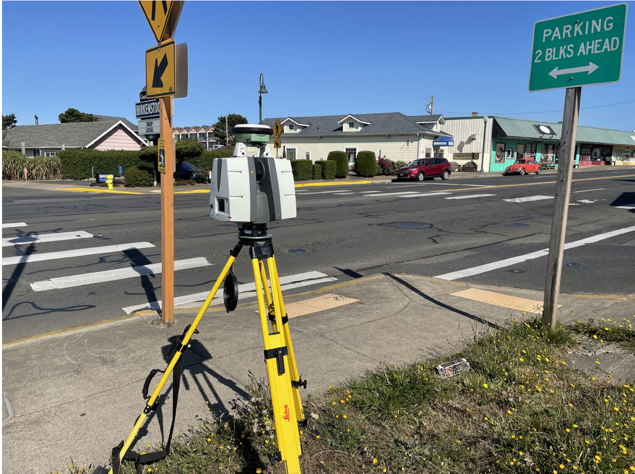
Figure 7.6: Terrestrial laser scanning data collection at a curb ramp.
