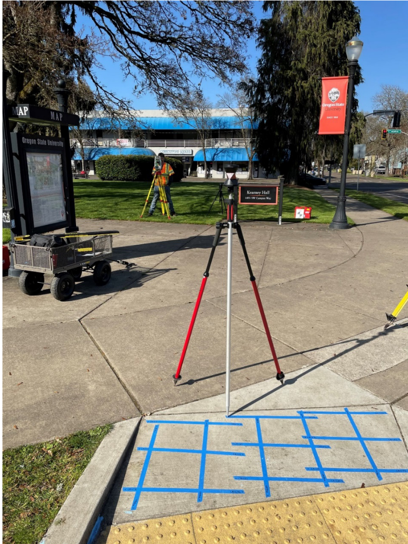
Figure 4.3: Total station measurement using Leica 360° prism with a bipod.
