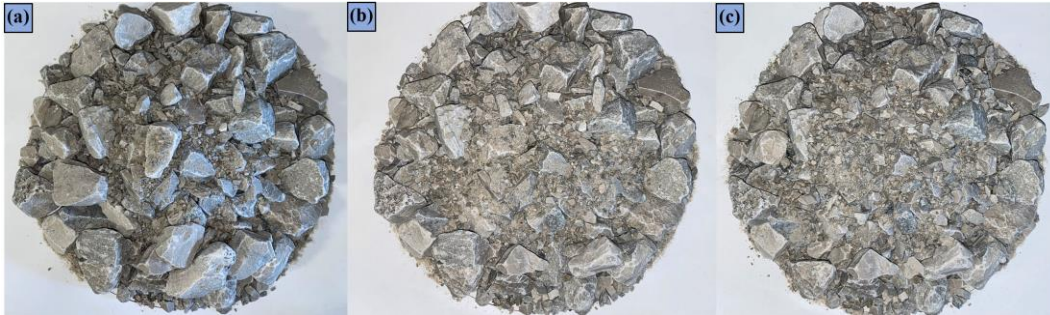
Figure 78. Ames Mine with increasing fines contents: (a) 5%, (b) 10%, (c) 15%
