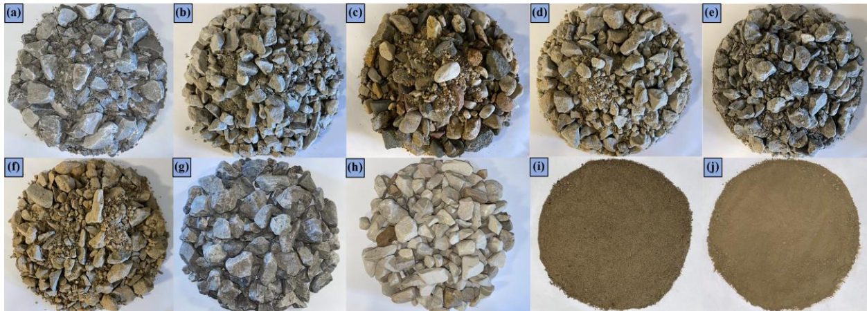
Figure 2. Materials used in the study: (a) Ames Mine, (b) Bethany Falls Limestone, (c) Crocker Pit, (d) Oneota Formation Dolomite, (e) Plano Quarry, (f) Weber Quarry, (g) Shambaugh Quarry, (h) Stone City, (i) Pottawattamie County CBIS (Council Bluffs Interstate System), (j) Plymouth County (95)
