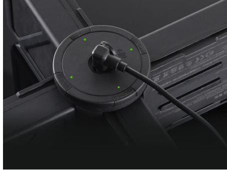
Figure 17. Photo. Charging Hub Status LEDs Display a Solid Green Light
