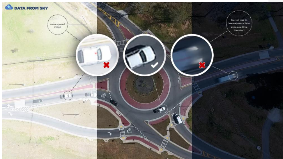
Figure 80. Three situations – not ok: too bright (left), ok: ideal (center), not ok: blurred due to low exposure time (right) Source: DataFromSky®
