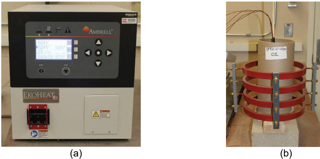
Figure 21. laboratory induction heating setup: (a) EKOHEAT 15/100C power supply; (b) 3.8 L fiber tube in laboratory coil (59)
