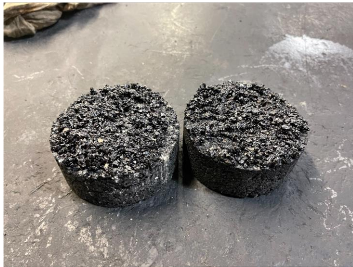
Figure 59. Damage form of CMA-B during interface shear test
