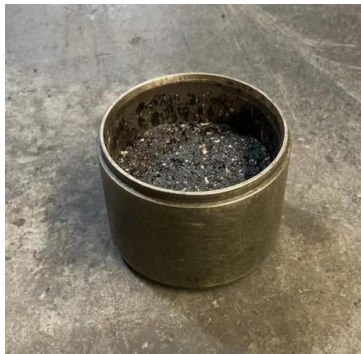
Figure 56. 3.8-cm-thick Marshall specimen
