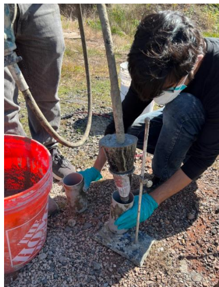
Figure 21. Inverted slump test
