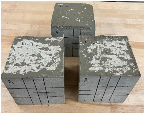
Figure 25. CSA cement cube samples for 3- hour testing
