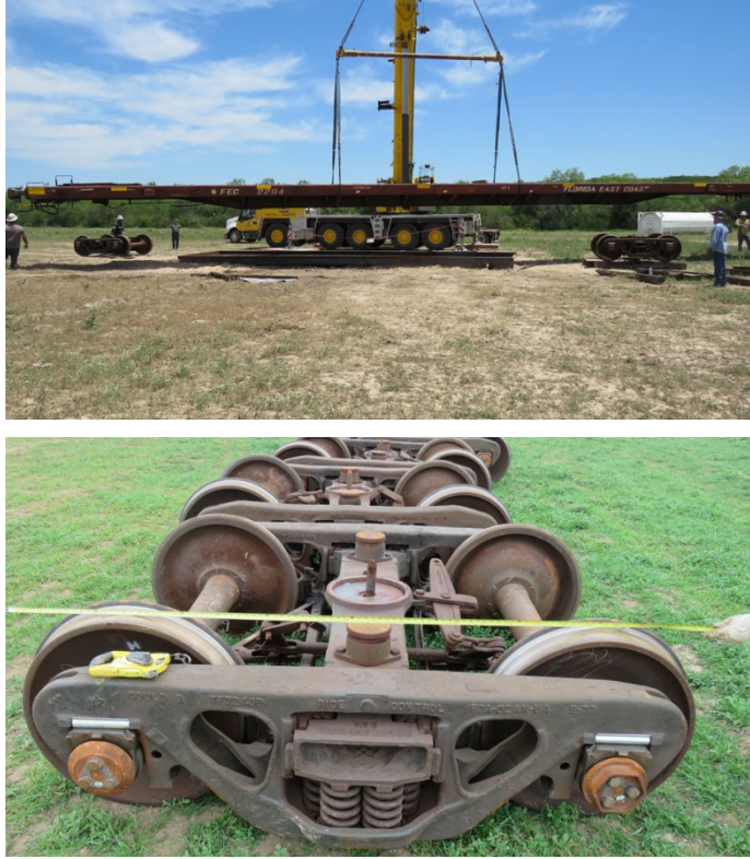
Figure 2. Flatcar Photographs (top: Flatcar Being Installed; bottom: Flatcar Trucks)
