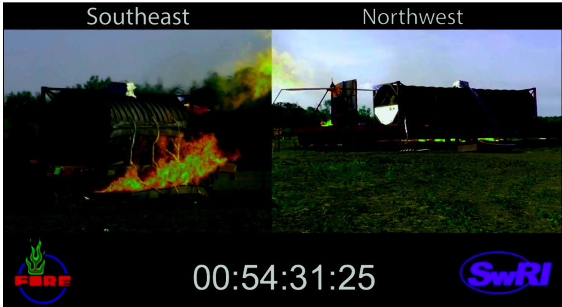
Figure 66. Jet Flame Geometry at Maximum Internal Tank Pressure (180 psig); Note how Horizontal the Jet is with Most of the Flame Off-Screen to the Left
