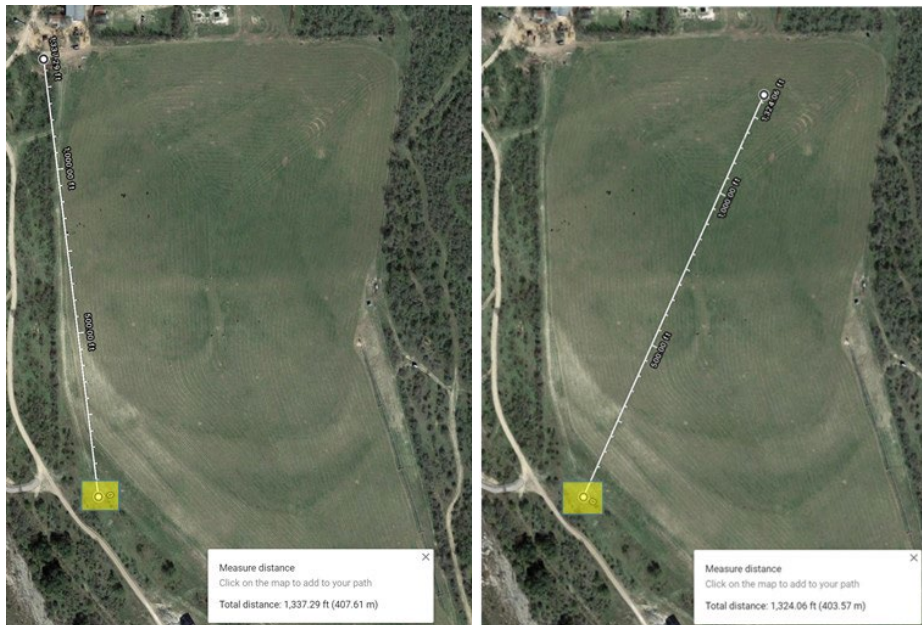
Figure 6. Location of Staff Bunker (yellow box) During Phase 2 Test (left: 408 m from Bunker to Propane Tank; right: 404 m from Bunker to Test Article)
