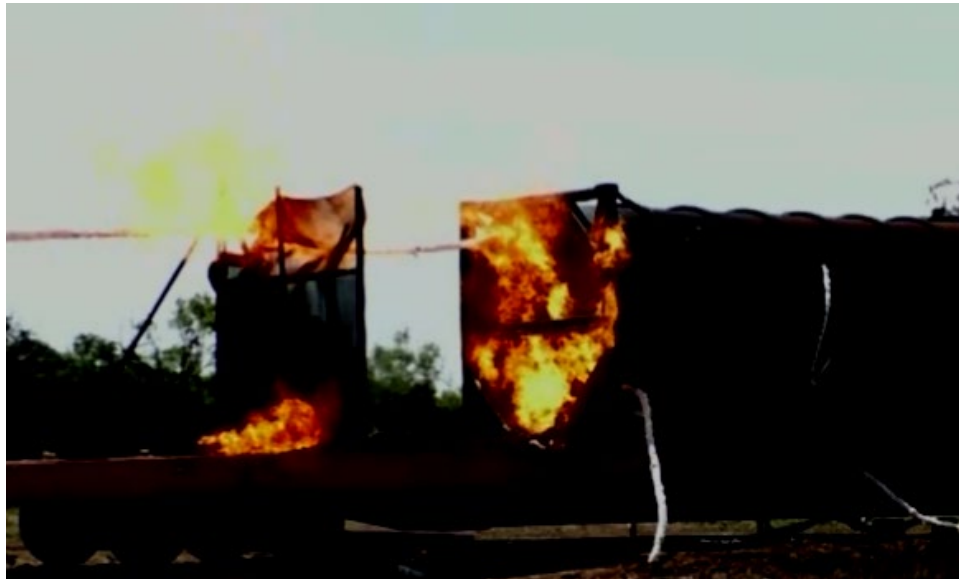
Figure 55. Typical Post-Test Piping Cabinet Fire Behavior [04:23:33]
