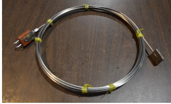
Figure 15. Weld-Pad Surface Temperature Thermocouple Probe
