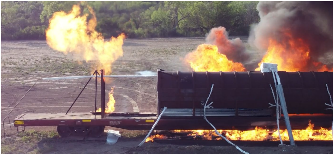
Figure 67. Jet Flame at Internal Tank Pressure of ~129 psig (view from drone) [~00:41:15]
