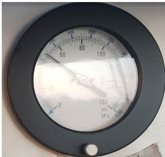
Figure 35. Pressure Gauge on Tank Indicating ~49 psig (337,843 Pa gage) 1 h Prior to Test
