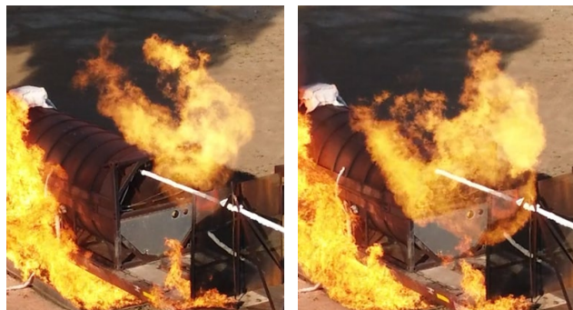
Figure 50. PRV Flame Comparison Prior to (left) and During (right) the Rapid Pressure Drop [~00:38:30]
