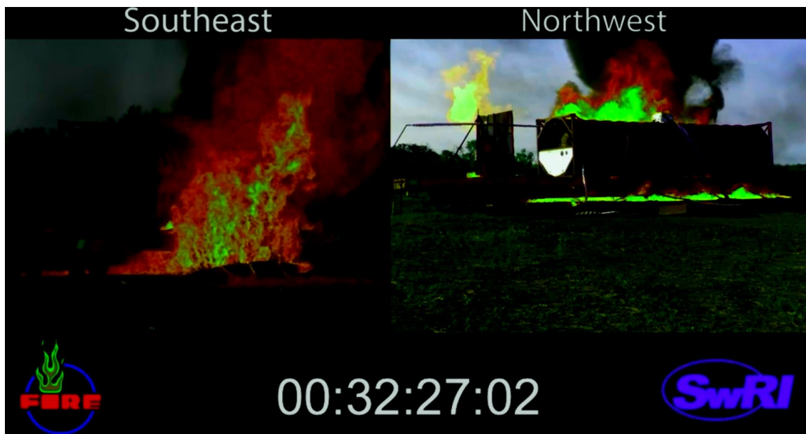
Figure 63. Jet Flame Geometry at Internal Tank Pressure of 114 psi (PRD setting)
