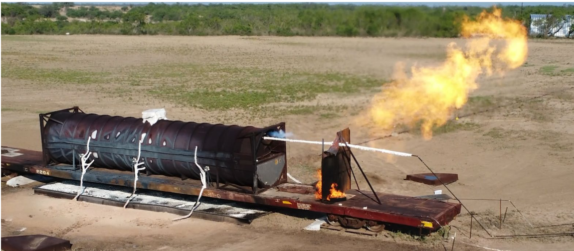
Figure 69. Jet flame at Internal Tank Pressure of ~180 psig [00:56:00]
