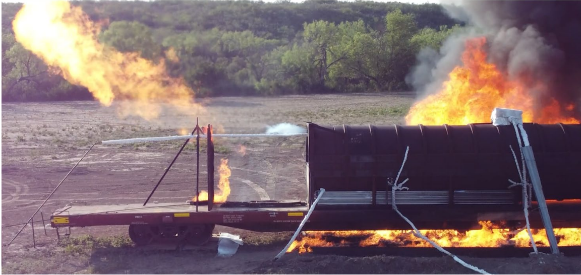
Figure 68. Jet Flame at Internal Tank Pressure of ~156 psig [00:46:52]
