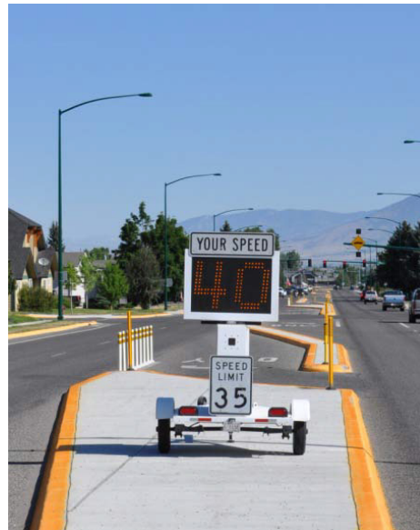
Figure 2.4: Example of trailer-mounted radar speed sign (Veneziano et al. 2012)
