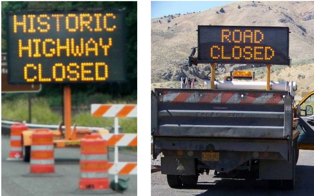
Figure 2.3: Examples of portable changeable message signs: trailer-mounted (left) and truck-mounted (right) (ODOT, 2018)
