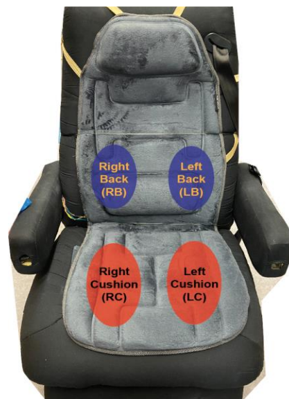
Fig 6. Active Seat with embedded Vibrotactile Motors
