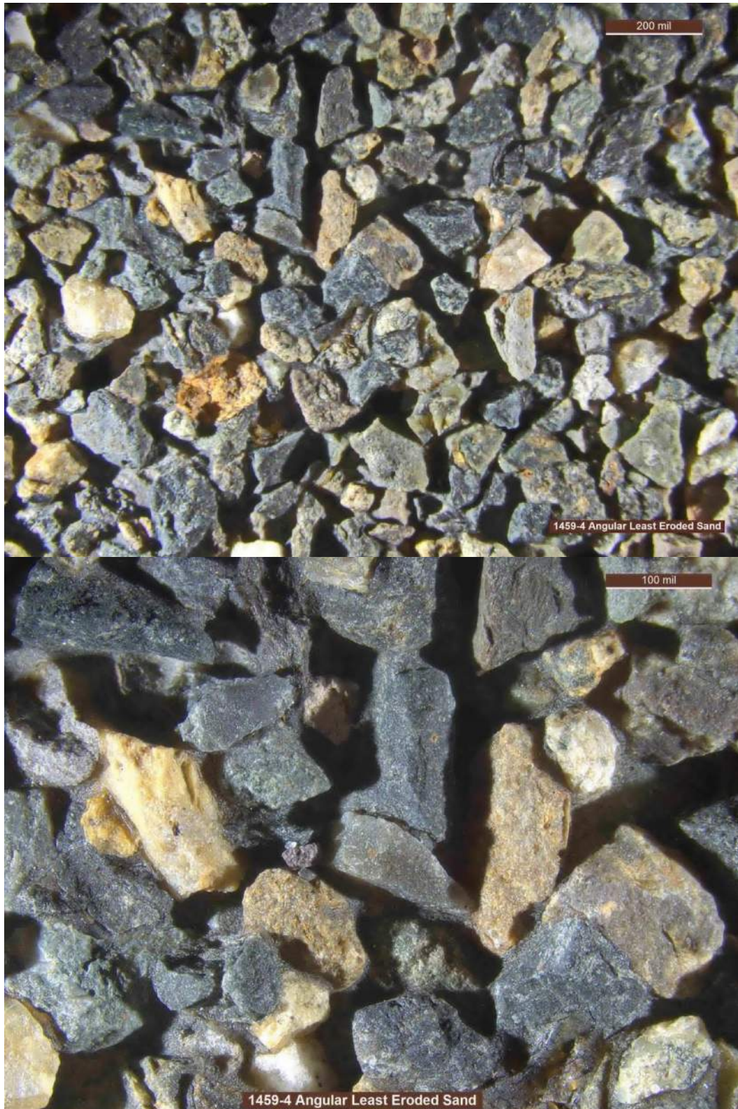
Figure C.20. Core 1459-4. Close-up views of the top surface show angular sand particles stand proud of resin (rarely visible). The texture is consistent with absence or minimal smoothing or erosion by traffic.
