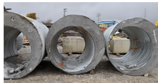
Figure 5: Cutting of a Culvert for Annulus Void Inspection (Left); Cut Surfaces of Hardened Grout (Right).
