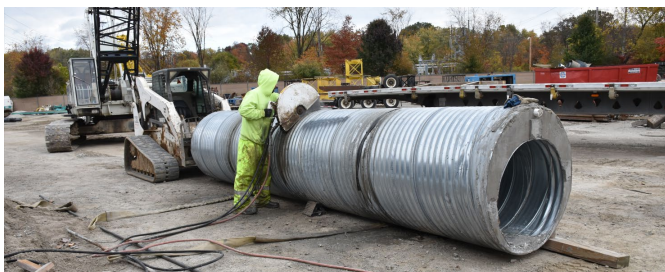
Figure 5: Cutting of a Culvert for Annulus Void Inspection (Left); Cut Surfaces of Hardened Grout (Right).
